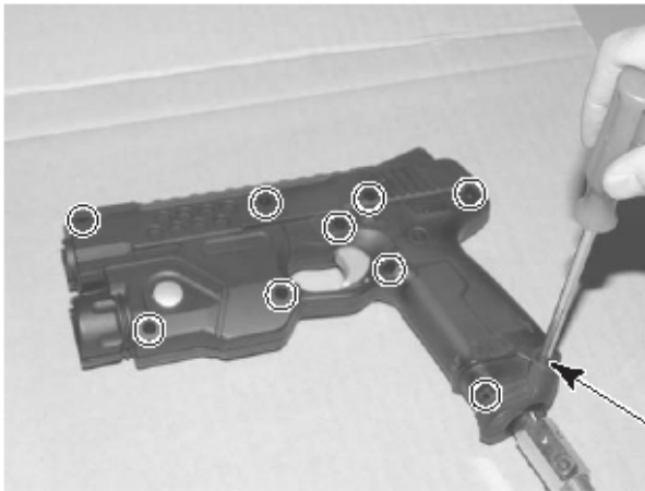
SCREW (10), black M3 x10, w/small flat & spring washers
